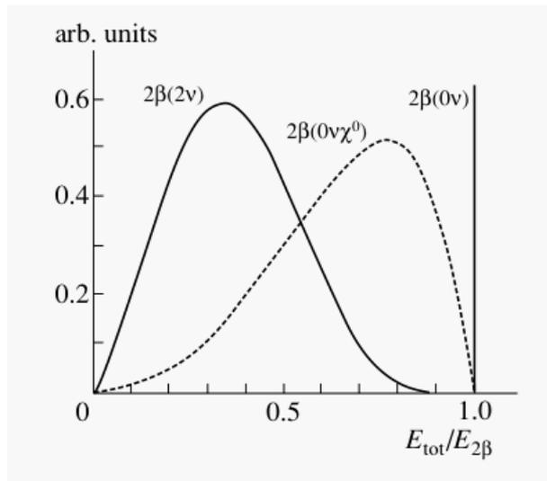
Figure 1.3 : The spectra of the summed electron energies, as a fraction of the total energy available in the decay. The standard model  $2\nu$  decay mode produces a continuous spectrum, while the  $0\nu$  mode is a delta-function at 1. Majoron emission can generate different spectra. From [5].
