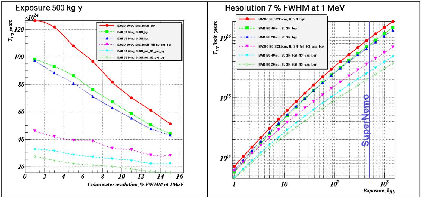
Figure 1.6: SuperNEMO half-life sensitivity for different detector layouts, background conditions and other parameters . Left: sensitivity as a function of the calorimeter energy resolution; Right: Sensitivity as a function of exposure.
