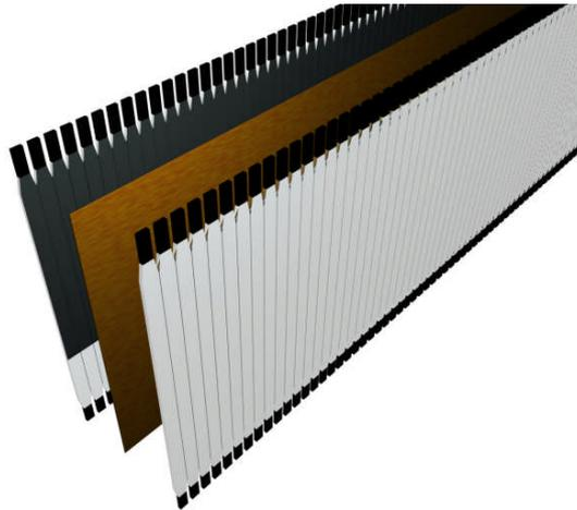
*Figure 1.5 : Schematic of the bar design, with walls of long scintillator bars read out at each end by PMT's. The source foil sits inside the same tracking volume as in the block design. The final detector would be a repeated array of such elements.*
