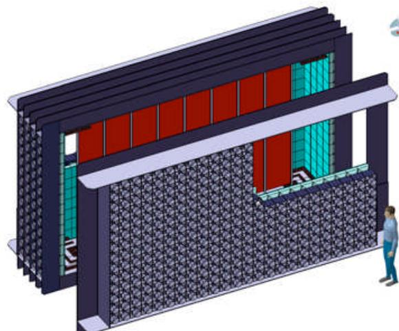
Figure 1.4 : schematic of a proposed SuperNEMO module showing the source foil (red) surrounded by a tracking volume and scintillator blocks read out by PMT's.
